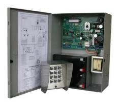
Crypto-Lock is a versatile, easily installed and operated single door access control system capable of operating virtually any electric or magnetic lock. Its microcontroller based design provides a high level of PIN security and comprehensive door control and monitoring functions. It is available with a surface mounted keypad, single gang mounted Smart Card Reader, or Smart Card Reader with keypad.
